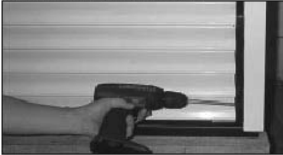
1. Unscrew four screws securing the Bottom Grill.
