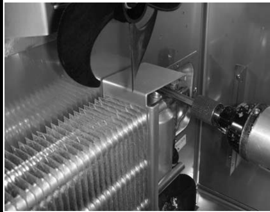
A.Remove the evaporator coil
