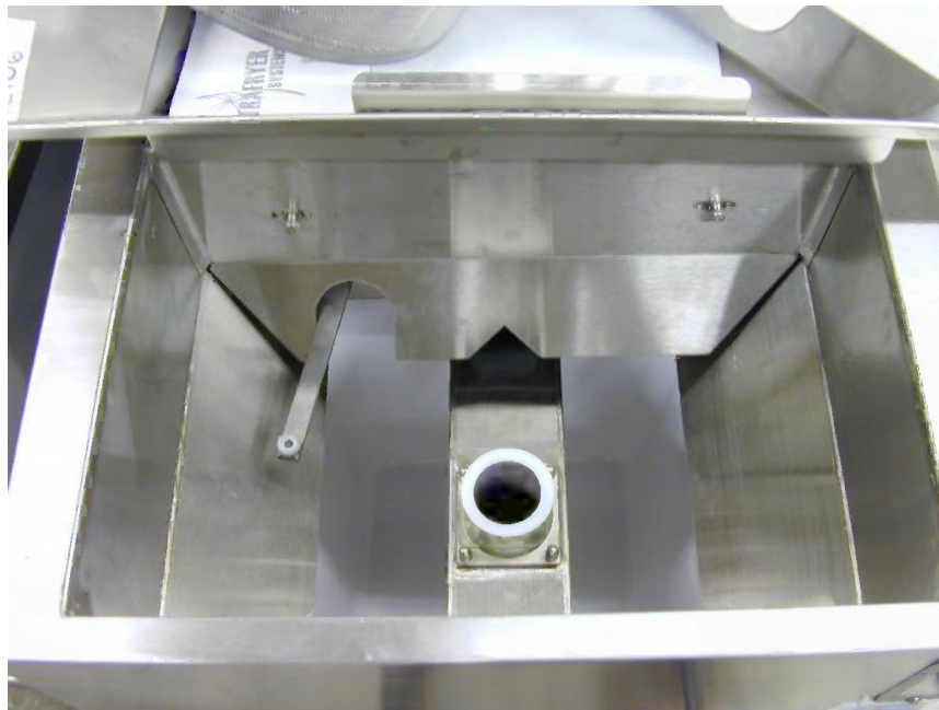
View Looking Down Inside of Sifter Area (shown with cover removed)
