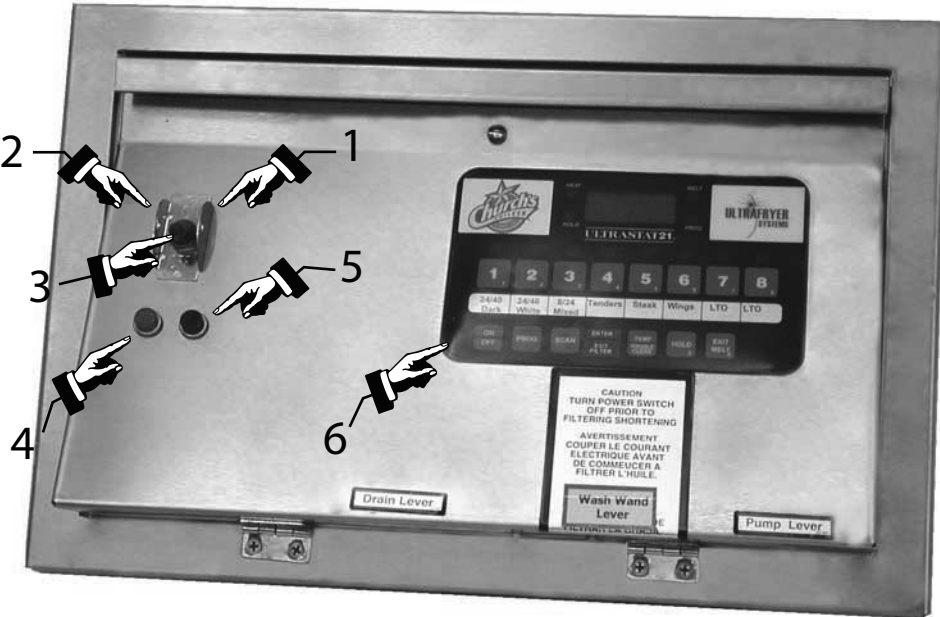
PAR-2-20F CE PANEL WITH DIGITAL TIMER
