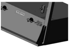
Attach all the legs to the base using 16 screws (2 screws per top support bracket). The nuts for these screws are permanently attached inside the base.
